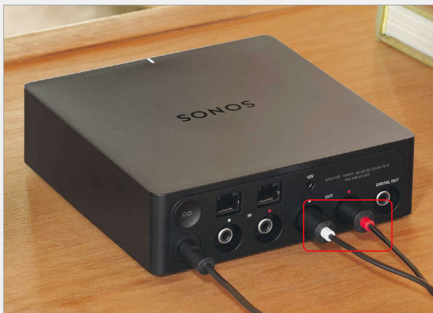
The Sonos Port can connect to a standard hi-fi system as well as Sonos speakers
