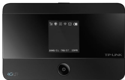
TP-Link's M7350 4G LTE MiFi router can connect up to 10 devices to 4G networks
