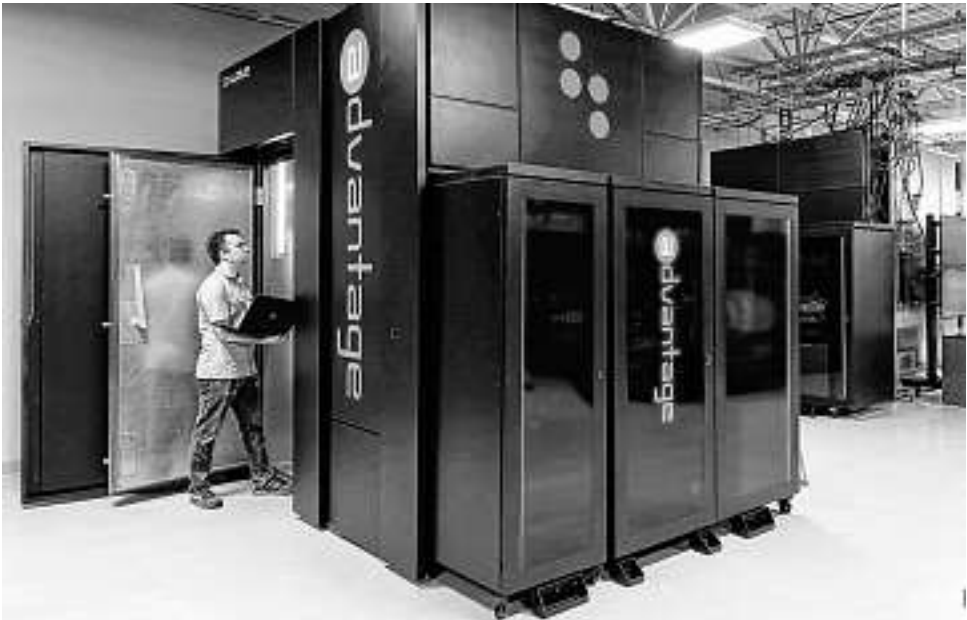
D-Wave's Advantage system uses quantum annealing, a form of quantum computing.
