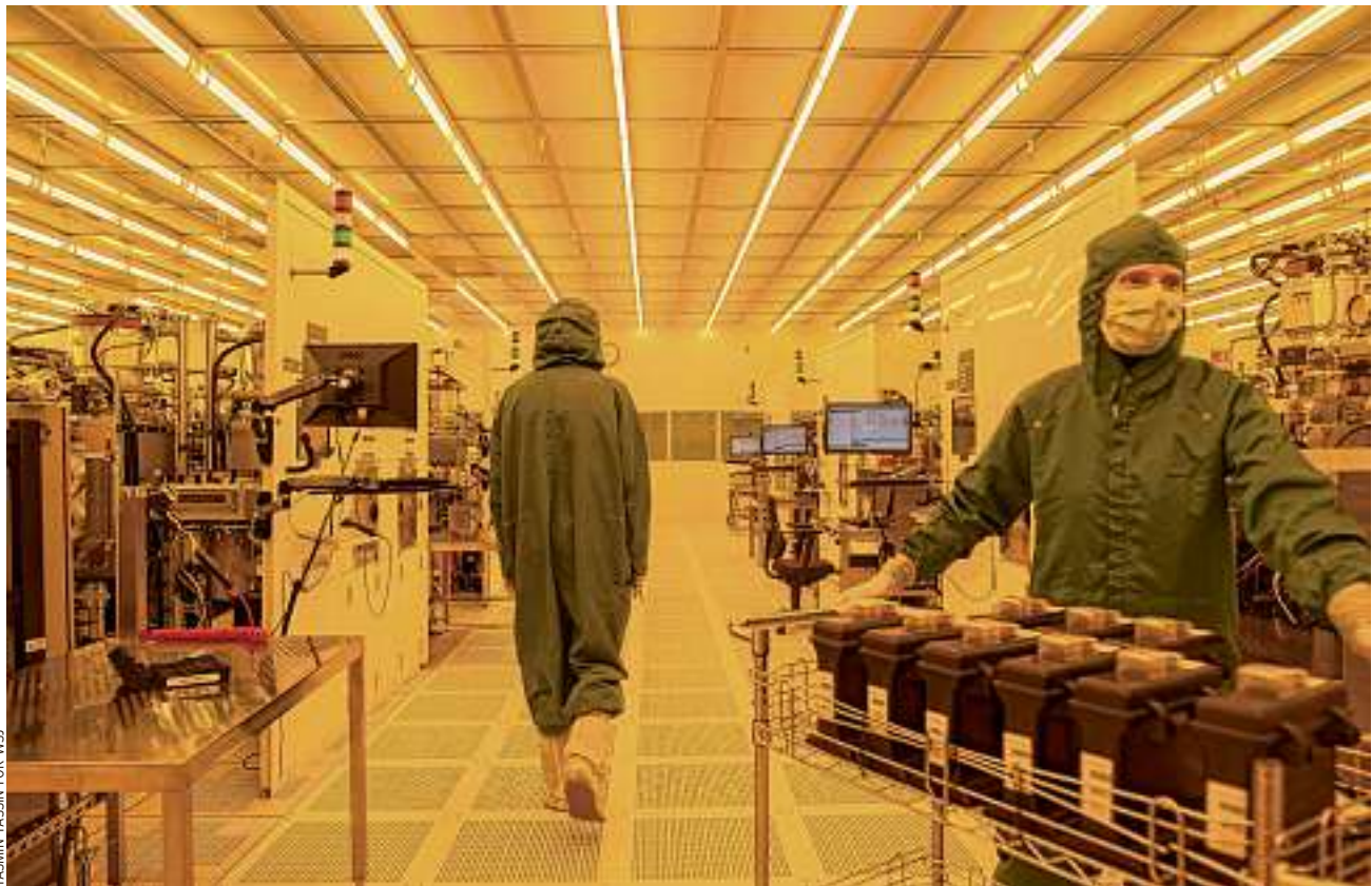
Hard-drive components that record information are made in vast clean rooms at Seagate's suburban Minneapolis factory.
