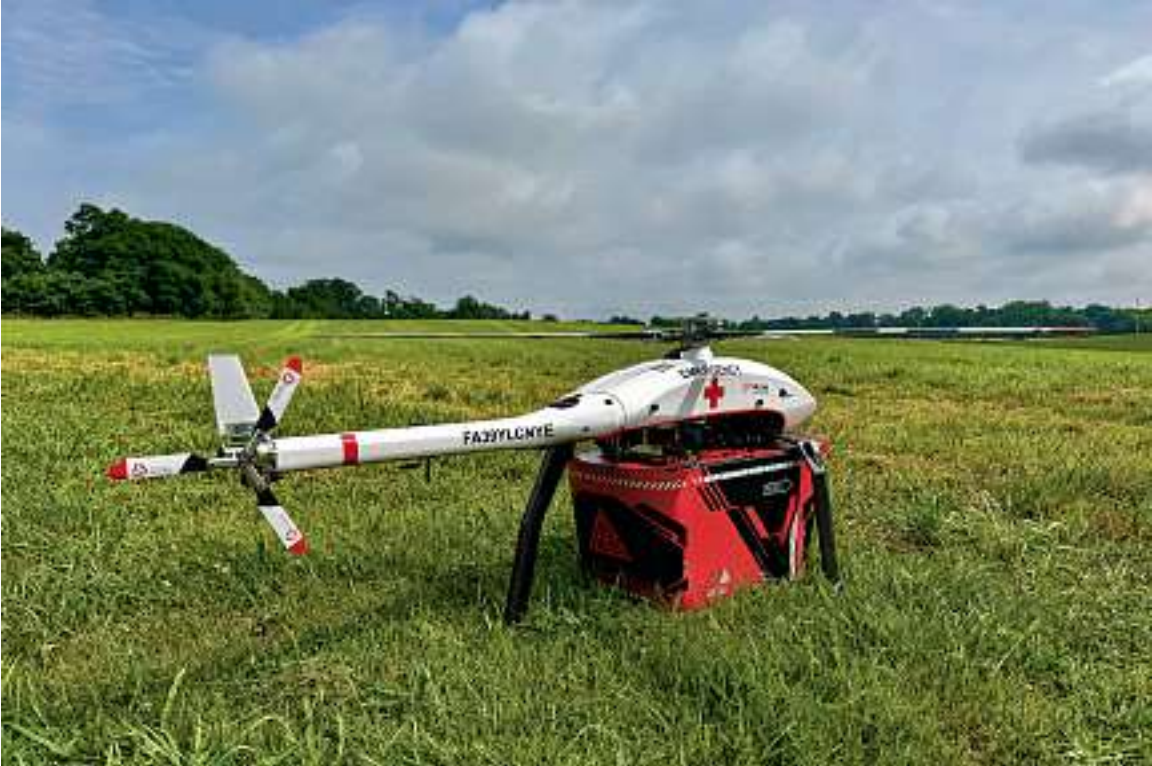
A drone with a cargo attachment, in an organ shipment simulation.
