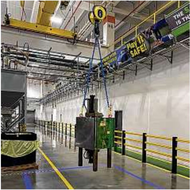
Eliminating forklifts reduced injuries in Whirlpool's factories. Below, Ipex designed its new factory to rely on overhead cranes and hand-pushed pallet jacks.
