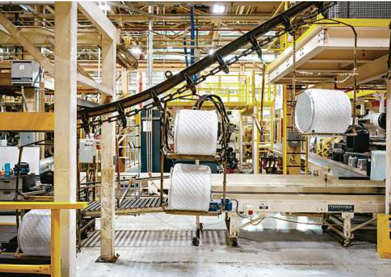
Whirlpool's factory in Clyde, Ohio, eliminated forklifts from its production area. Conveyor belts do some of the work.
