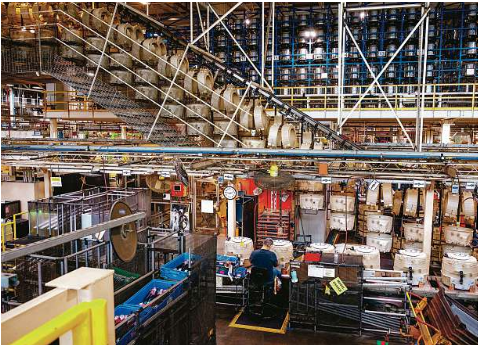
Eliminating forklifts reduced injuries in Whirlpool's factories. Below, Ipex designed its new factory to rely on overhead cranes and hand-pushed pallet jacks.
