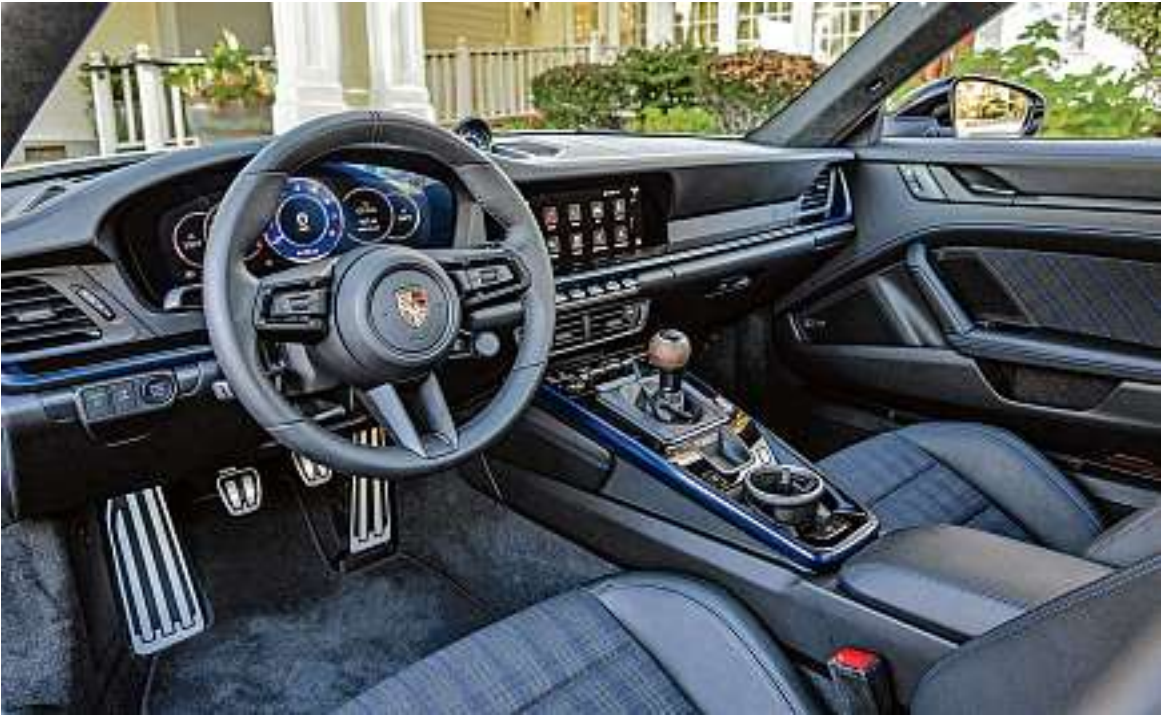
The Carrera's clutch pedal throw is short and well-weighted—and ideally spaced for heel-and-toe downshifting.
