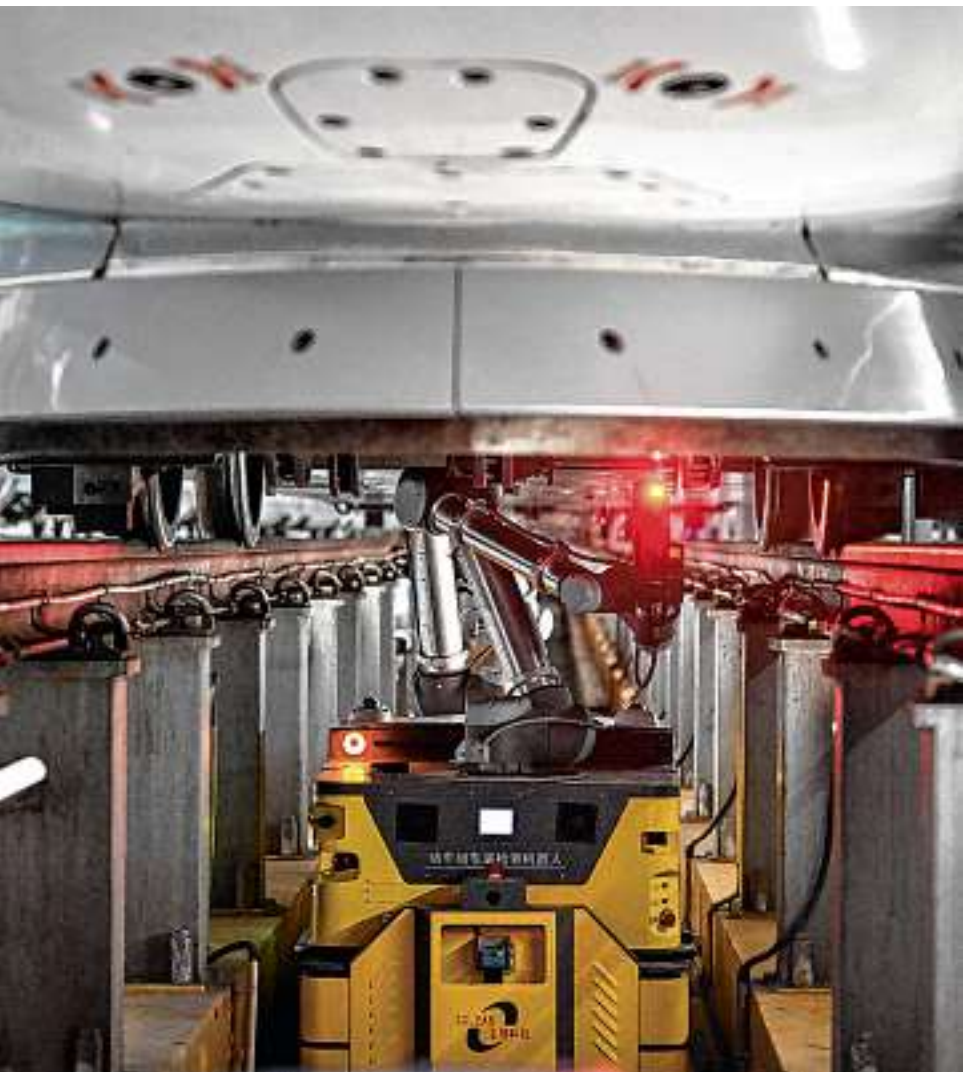
A robot inspects a bullet train at a high-speed train maintenance base in Beijing.
