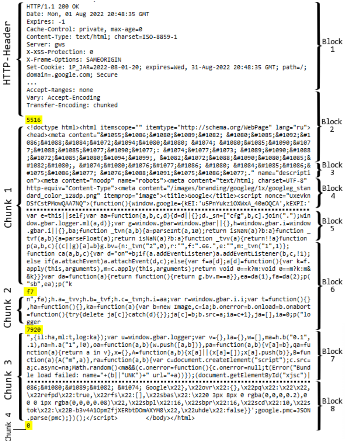
Fragmentation of a web document during transmission at the HTTP and TCP levels
