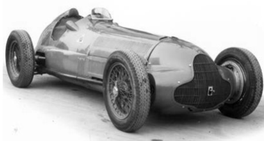
In 1947, Alfa Romeo updated one of the existing Type 312 chassis, installing a 4.6-litre, supercharged V12 and giving it revised bodywork, more akin to its then successful Type 158
