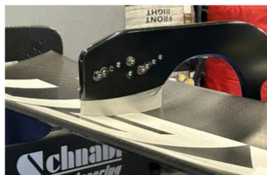
The rear wing on the Porsche 911 GT3 R is adjustable, although each GT3 manufacturer is given a maximum permitted wing angle to use
