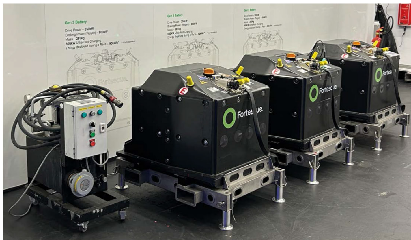
Fortescue's Formula E batteries on display in the paddock at the London E-Prix. The cells within these packs need to be replaced at the end of each season as they are being pushed to their limits
