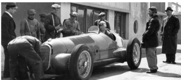
As rolled out for the 1937 season, the Type 12C-37 shows its very narrow central frame, a characteristic that did not serve it particularly well
