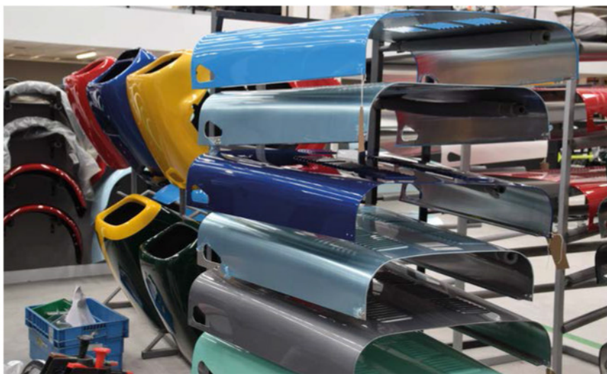
To keep costs under control, carbon fibre is not used on the bodywork, even of the higher spec racecars. All models can come in pretty much any colour you desire as the factory is equipped with its own in-house paint shop
