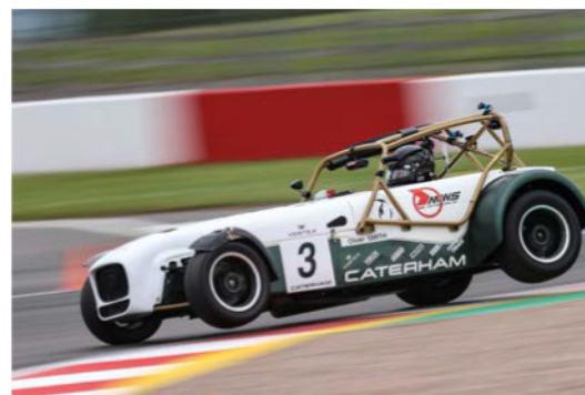
The full-race 420R uses a Sadev six-speed, sequential gearbox with manual shift, but still retains much of the simple design philosophy of the other racecars, including outboard suspension
