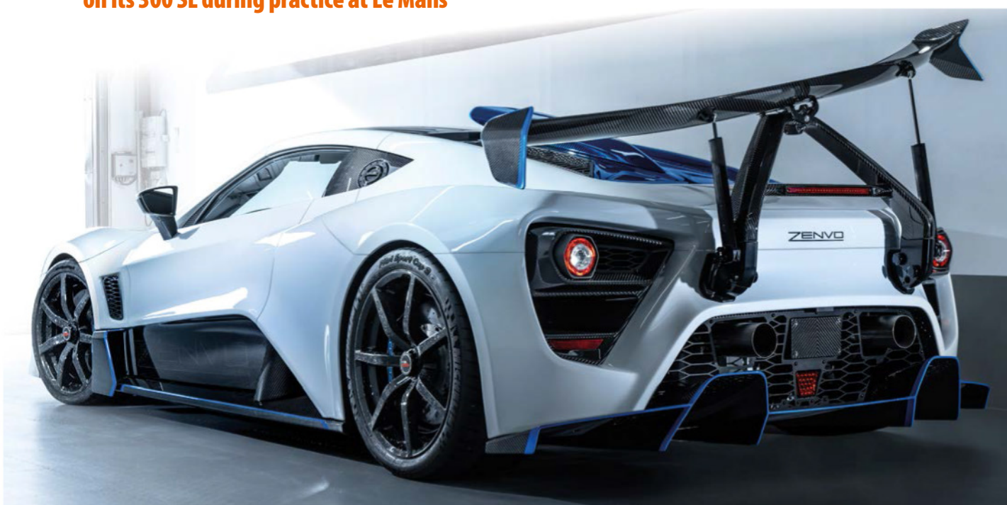
Danish supercar manufacturer, Zenvo, has developed a distinctive active aero system for its TSR-S road car. The rear wing tilts around corners, changing the lateral angle of attack by up to 20deg
