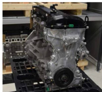
The 2.0-litre, 180bhp Duratec unit that's used in the top-level Seven UK championship for 420R racecars. These are fitted with bespoke pistons and camshafts to ensure all engines racing are exactly the same spec
