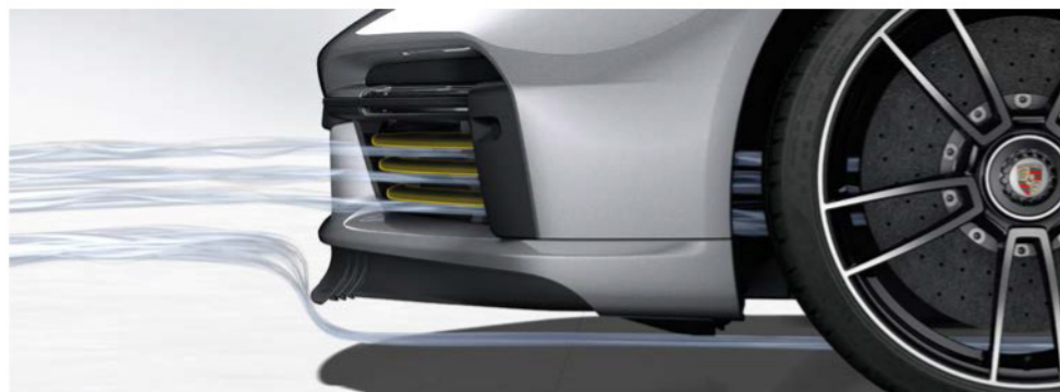
Porsche employs active cooling flaps and front splitter on the latest version of the 911, both controlled by electric servo motors
