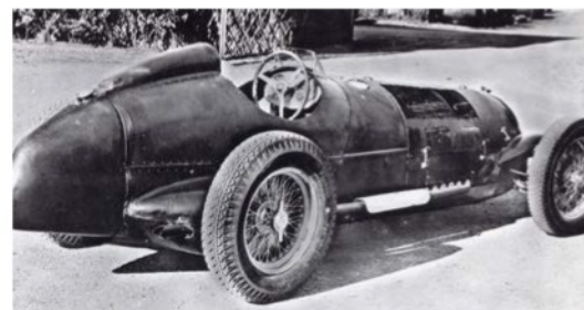
The narrow central frame passing under the machinery kept Alfa from making the best of its 12C-37, as this rear view suggests
