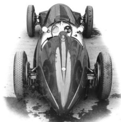
The restored and re-bodied Type 312 kept the now outdated swing axle rear suspension but wore the latest Pirelli Stelvio racing tyres
