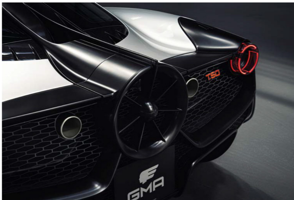
The moveable aerodynamic devices from Brabham's F1 1978 fan car are clear to see in the same designer's T.50 road car
