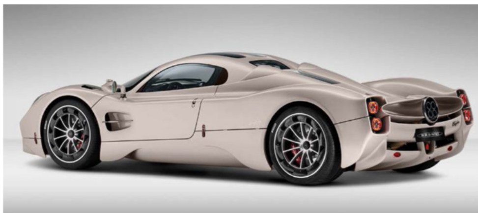
The V12, twin-turbocharged Pagani Utopia is equipped with an active aero device on the rear that, according to the Italian manufacturer, combines with the electronically controlled suspension to produce 'maximum stability in every driving condition'
