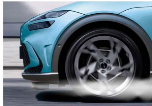
Hyundai's Active Air Skirt controls air turbulence around the wheels at high speed. Tests on an SUV saw drag coefficient reduce by 2.8 per cent
