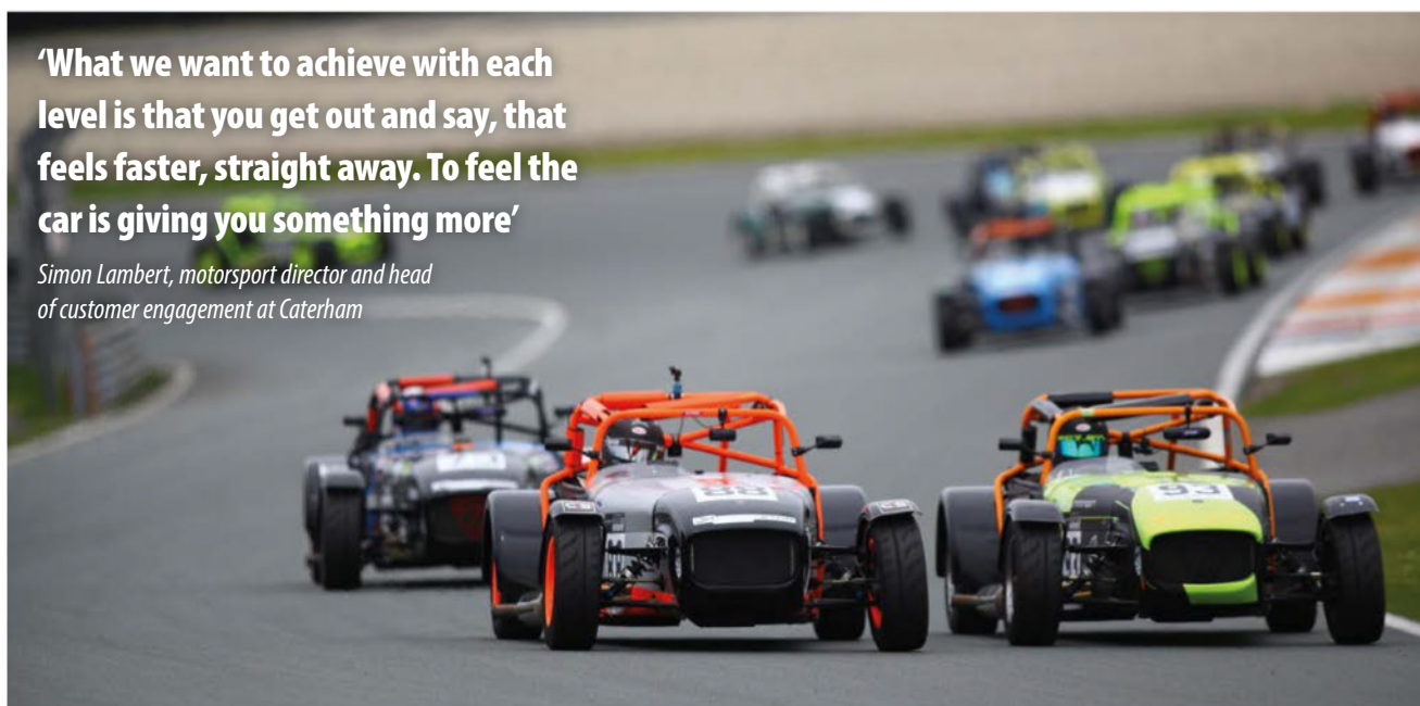
With high drag aero that promotes slipstreaming, Caterhams racing are always exciting to watch. The 270Rs (shown) run without windscreens and lights and with a wider track front suspension
