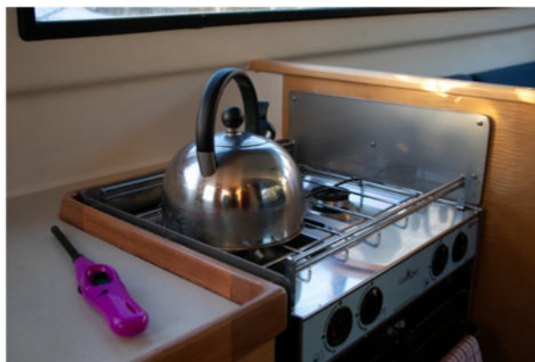
A gas hob with a suitable surround to meet the rule that all surfaces within 200mm of the flame be non-combustible.
