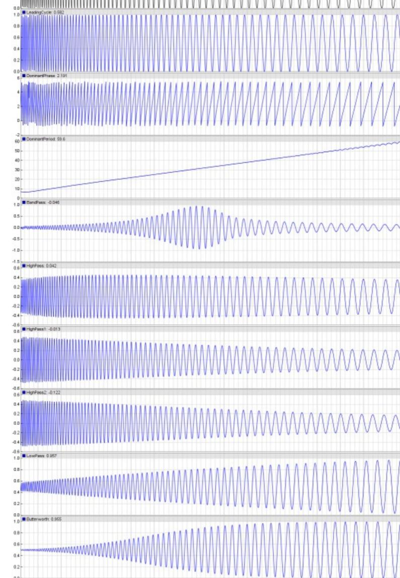
Output of some spectral filters applied to a sine chirp with a period from 5..60 bars (generated by the **Filter** test script); top to bottom: **Data**, **Leading Cycle**, **DominantPhase**, **DominantPeriod**, **BandPass**, **HighPass**, **HighPass1**, **HighPass2**, **LowPass**, **Butterworth**.
