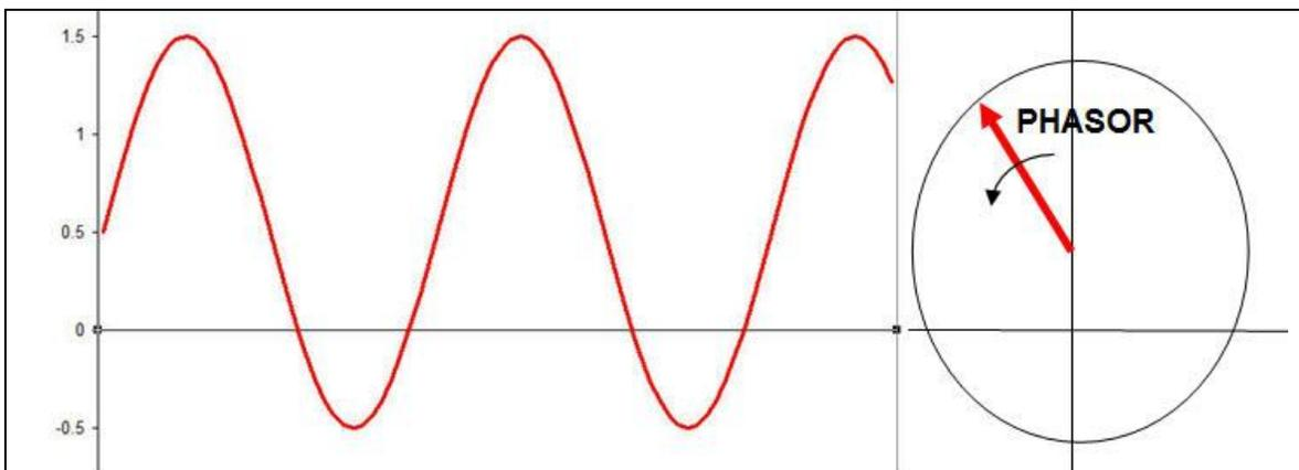
**Figure 5. Phasor Generation of a Sinewave in a Trend**
