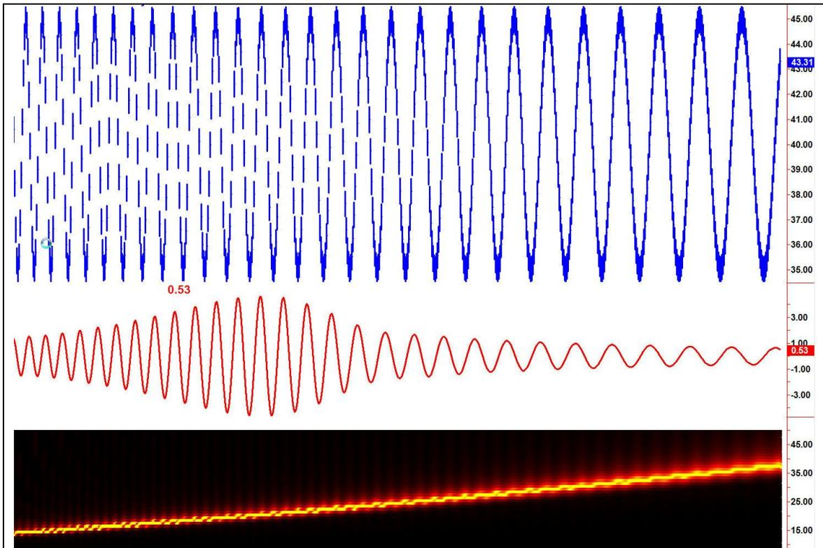
**Figure 2. A Chirp Waveform Demonstrates the Selectivity of the Bandpass Filter**
