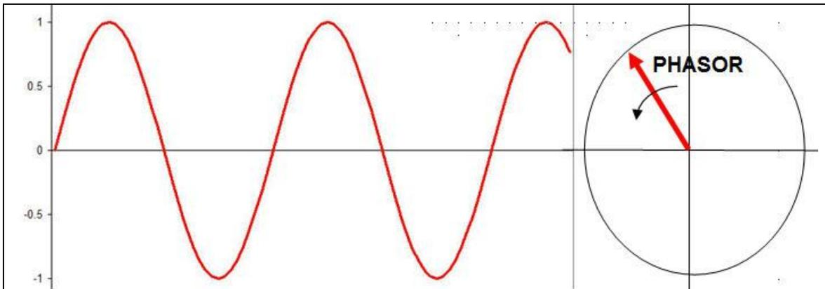
**Figure 4. Phasor Generation of a Sinewave**
