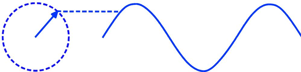
**Figure 9. The Relationship Between the Phasor and the Time Domain Waveform**
