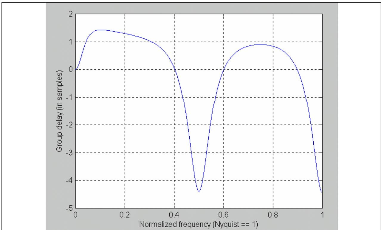
**Figure 5. Zero Lag IIR Filter Lag Response,  $\alpha = 0.2$**
