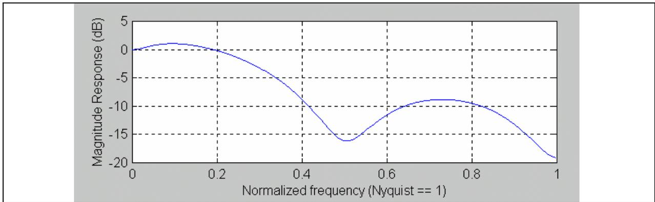
**Figure 4. Zero Lag IIR Filter Amplitude Response,  $\alpha = 0.2$**
