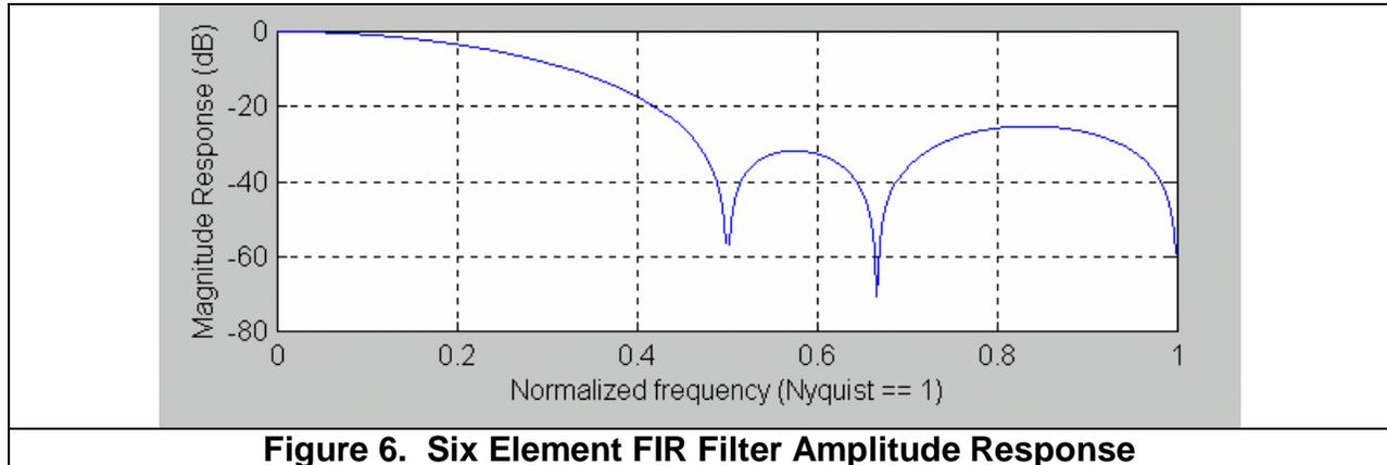
**Figure 6. Six Element FIR Filter Amplitude Response**
