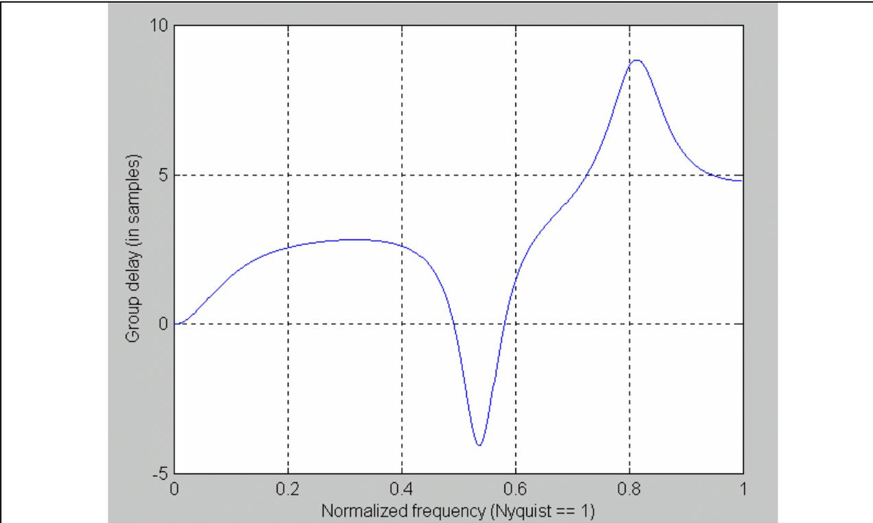
**Figure 8. Zero Lag FIR Filter Lag Response**
